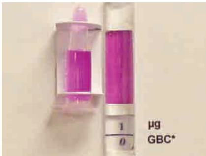
Fig 3. Close-up of Skin Contamination System showing color Comparison and the collection of 1 µg sample
