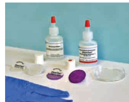
Fig 1. Surface Wipes for Chromium VI showing two unexposed wipes exposed to Chromium VI on the right.
