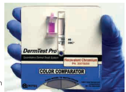
Fig 2. System for Determining Skin Contamination of CrVI
